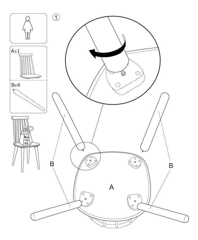
Check that legs are properly tightened on regular basis.
