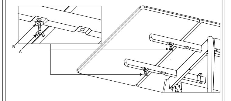
STEP 4: Insert the wing screw on Table side, but before tighten it, push the leaf panel until no gap visible between leaf and top panel, then please ensure all wing screw fully tightened.
