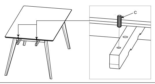
STEP 2: Carefully align holes on leaf panel with dowel as shown below. Please ensure that dowel fully attched on leaf panel and extension slide.
