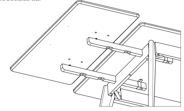
STEP 3: Please tighten the wing screw (using hand) on leaf panel first.
